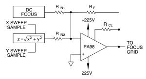
perhaps automatic focusing circuitry might be used to generate this potential. The dynamic correction is generated from the sweep voltages by calculating the distance of the beam from the center of the display.
